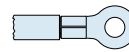
Lug Terminal for Attaching Receptacle Covers to a Panel with a Screw
