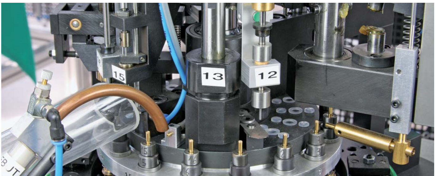
In-line mechanical and electrical checks are carried out on the assembly machine
